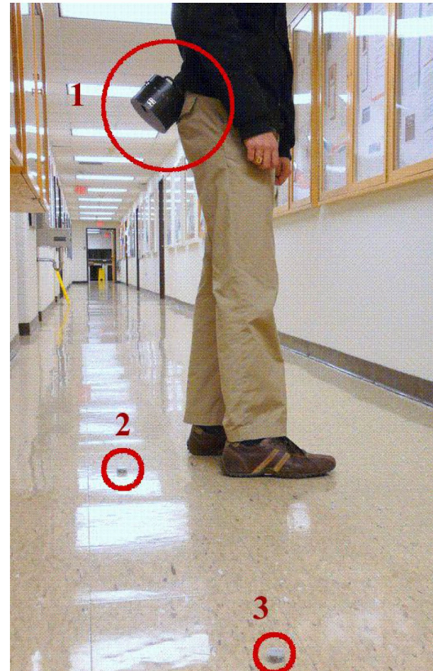
(c) A firefighter equipped with a smart dispenser, and two breadcrumbs dropped on floor.
